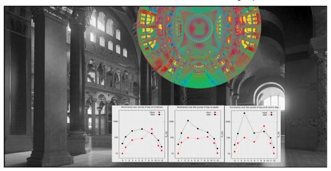
Fig. 5. Exemplary simulation results. Numeric data is stored in tabular form and visualised in diagrams (bottom) or false colour representation (top). Imagery visualises human perception models (background). © Authors.
