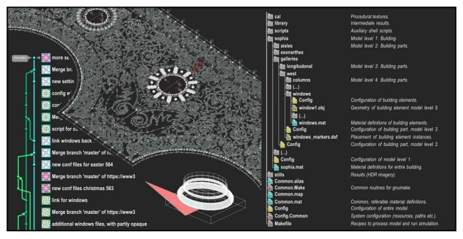
Fig. 4. The simulation environment combines the geometry of the reconstruction model (top left) with material models and configurations in a file system tree (right, Grobe et al., 2020). All data except images are stored in clear text formats allowing version control (left). Objects are placed as instances (bottom centre). © Authors.
