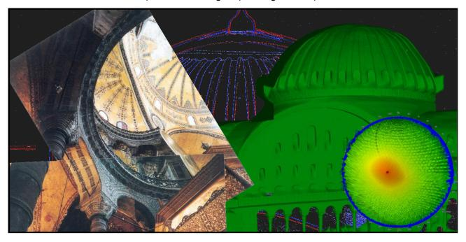
Fig. 2. Exemplary data from the Hagia Sophia project. Digital and analogue images from the photographic documentation (left). Digitised plans from a building survey (background). Triangular geometry derived from structure from motion techniques (right). Data from goniophotometric measurements (bottom right). © Authors.
