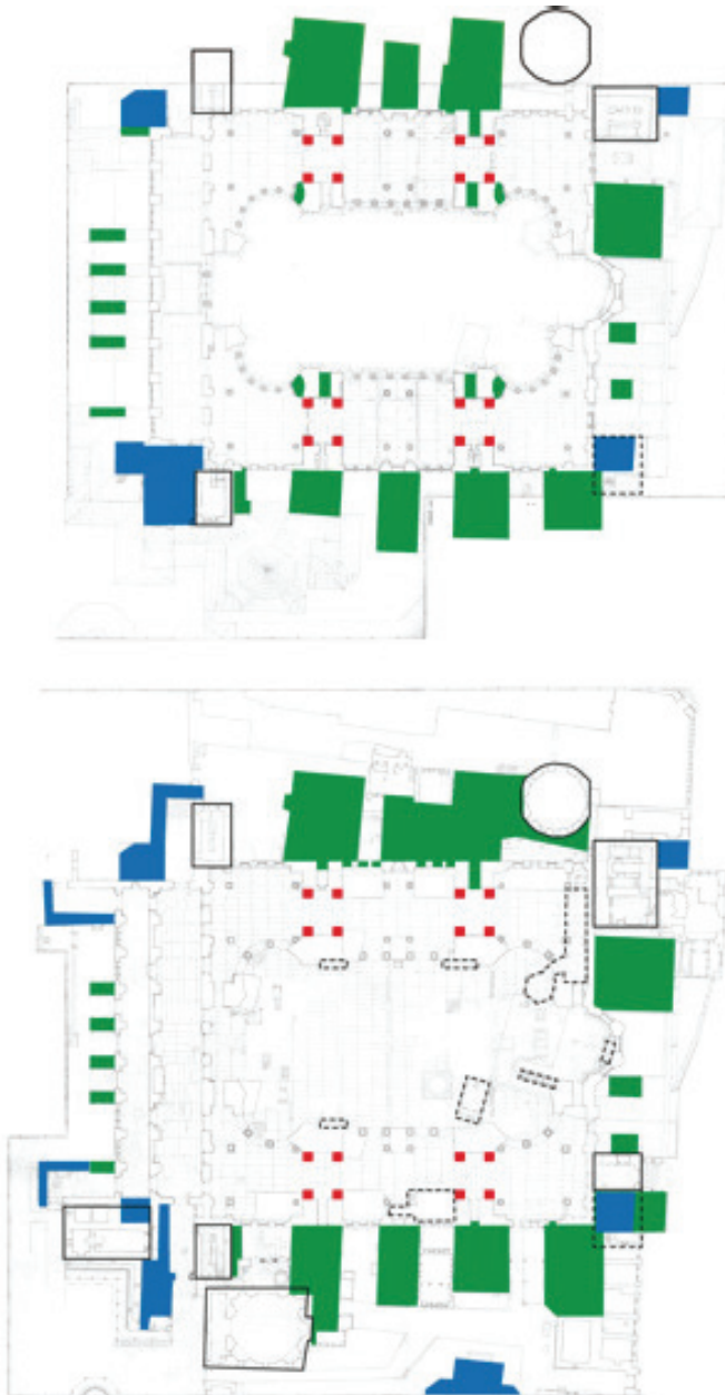
Figure 5. Daylight obstructions and later additions at the galleries (top) and the ground floor (bottom): structural reinforcements before (red) and after 562 (green), Byzantine (black) and Ottoman (blue) exterior additions, and later additions.
