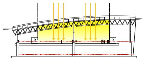
Figure 2: Daylight for central areas via skylights.
