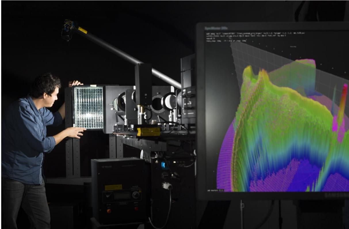
Figure 6: Daylight redirecting panel mounted on the scanning goniophotometer.
