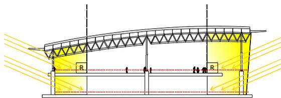
Figure 1: Daylight for perimeter zones via facades.
