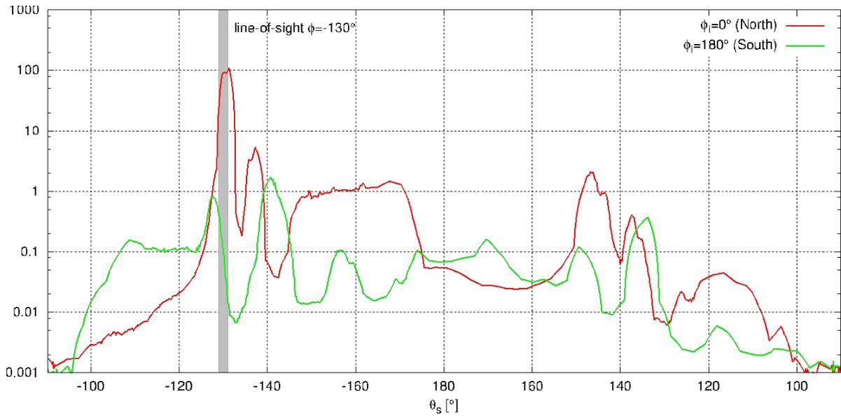
Figure 9: Profiles through distributions for incident direction  $\theta = 50^\circ$ ,  $\phi = 0^\circ$  (North, red) and  $180^\circ$  (South, green).
