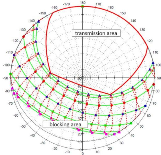
Figure 5: Sunpath with overlaid directions where sunlight is blocked (South) or transmitted (North).
