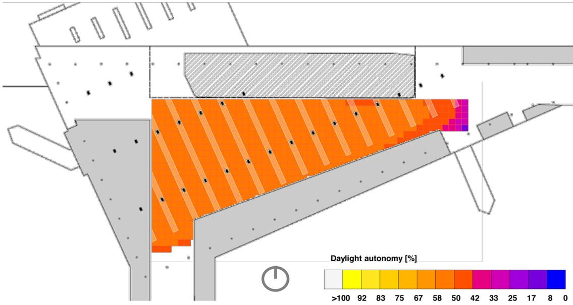
Figure 14: Daylight Autonomy DA for the Transborder Departures Level.
