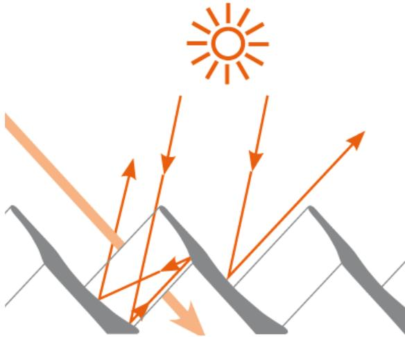
Figure 4: Embedded micro louver: principle of selective transmission.
