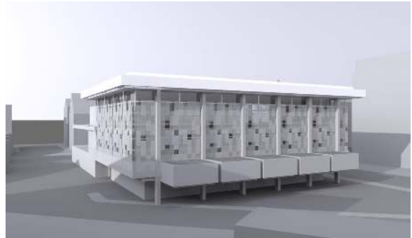
Figure 4: Several layers of fabrics in front of the glazing, R=0.25 , T=0.50 .
