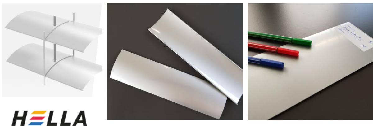
Figure 38: Round robin test system HELLA outdoor venetian blind ARB80. Product image (left; © HELLA Sonnen- und Wetterschutztechnik GmbH), test samples of shaped slats (center), sample of base material (right).
