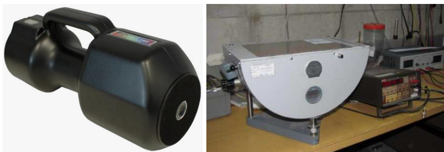
Figure 18: The Light Tec Mini-Diff V2 and a Carl Zeiss in-plane measurement goniometer for the characterization of base materials
