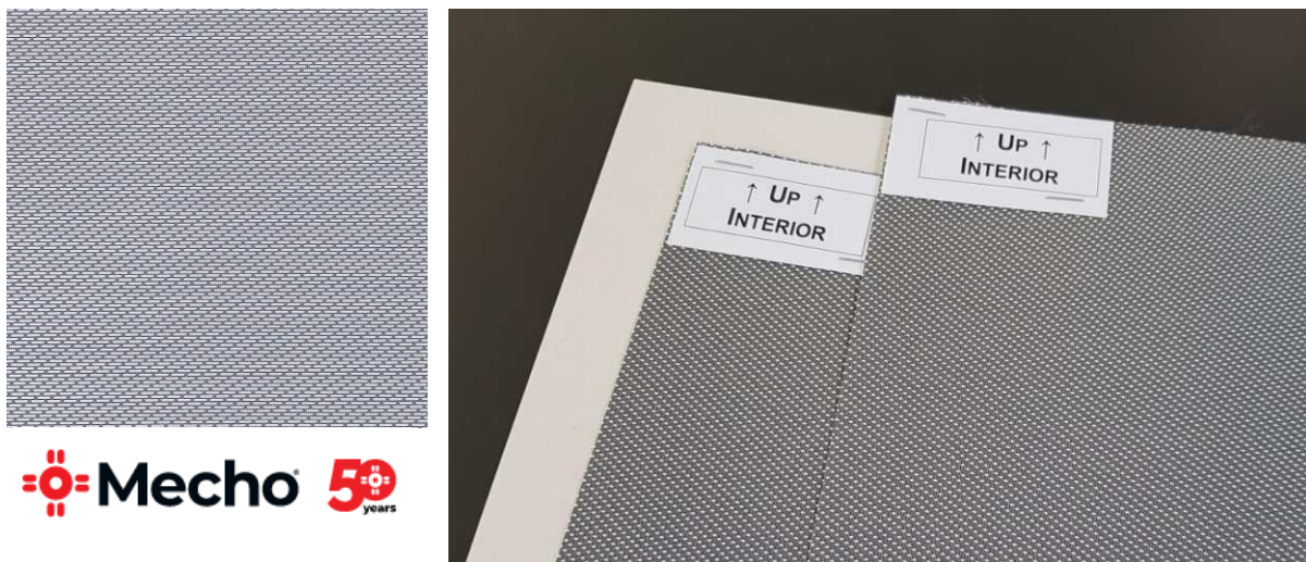
Figure 40: Round robin test system MechoShade interior textile roller blind. Product image of exterior surface (left; © MechoShade Systems, LLC.), interior surfaces of test samples (right).
