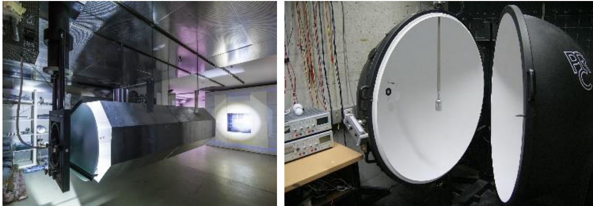
Figure 21: Devices to measure direct-hemispherical transmittance: artificial sun (left) and integrating sphere (right).
