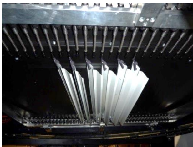
Figure 13: Slat turning device for venetian blind systems on the goniophotometer allowing to vary slat angle and slat distance
