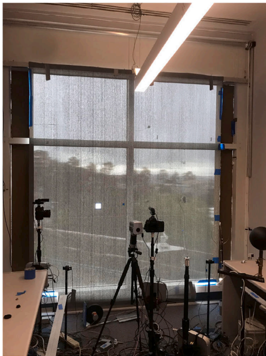
Fig. 19. Indoor view of the LBNL testbed office looking toward the south-facing window with the MS6216 roller shade fabric. The small square cut out is located in the lower left window at seated eye height. The gaps between the face of the window glass and the shade were blocked off on each side of the shade to simplify the simulation model. Unshaded portions of the window on the side were also blocked off. The electric lights (shown as “on” in this photograph) were turned off. Source: LBNL. (For interpretation of the references to color in this figure legend, the reader is referred to the Web version of this article.)
