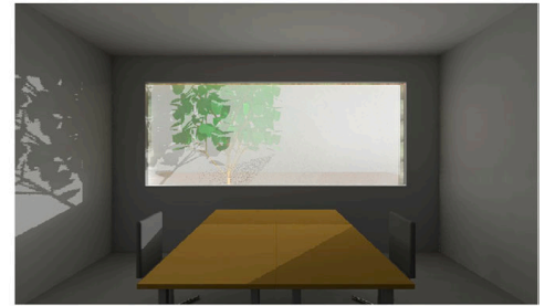
Fig. 8. Renderings of a scene with and without peak extraction to represent specular transmission through a fabric shade with about 2% openness. Source: Bartenbach GmbH. (For interpretation of the references to color in this figure legend, the reader is referred to the Web version of this article.)
