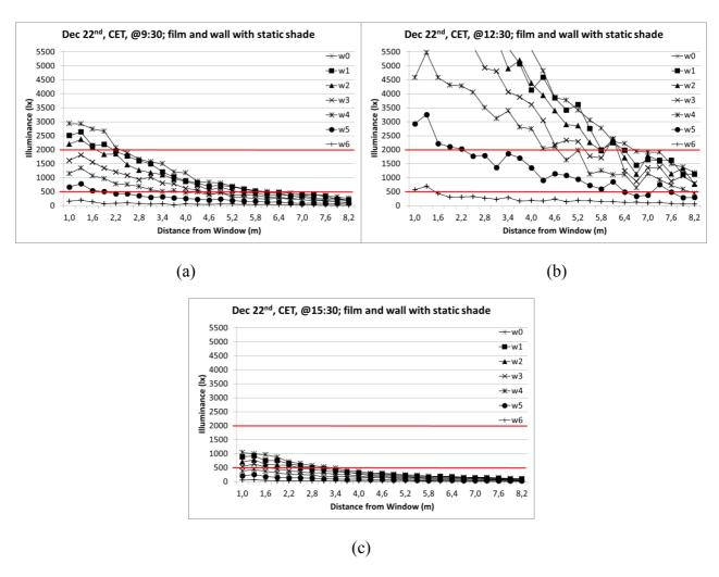
Fig. 15. Illuminance distribution at (a) 9:30, (b)12:30 and (c) 15:30 in the winter solstice.
