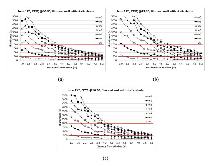
Fig. 14. Illuminance distribution at (a) 9:30, (b)12:30 and (c) 15:30 near summer solstice.
