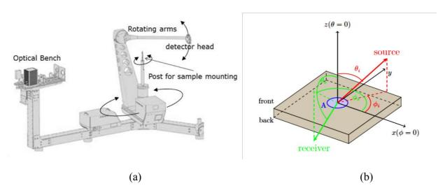
**Fig. 2** (a) Sketch of a goniophotometer; (b) Transmissive sample with source direction  $(\theta_i; \phi_i)$ , receiver direction  $(\theta_s; \phi_s)$  and sampling aperture A.
