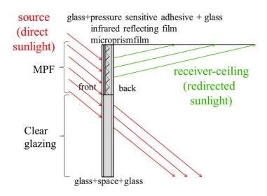
**Fig. 3.** Schematic section of a MPF and daylight redirection.
