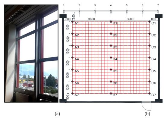
Fig. 1 (a) Window configuration; (b) Measurement points and sensor plane (the red grid).
