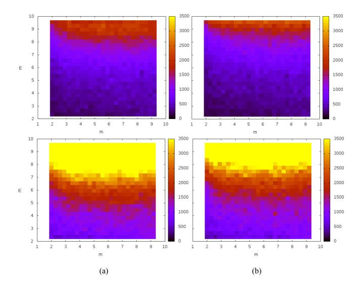
**Fig. 16**. Illuminance maps for (a) drc 2 and (b) w4 with static sunshade at 9:30 (upper row), and at 12:30 (lower row) near the spring equinox.
