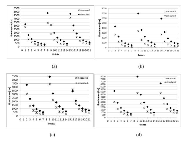
**Fig. 5.** Comparison of measured and simulated results for (a) a sunny, (b) a cloudy (c) and (d) partly cloudy days.
