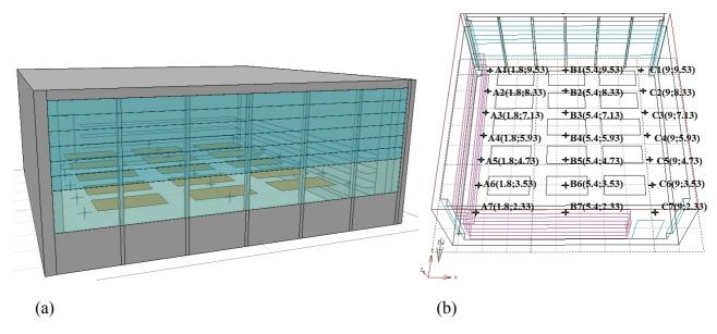
**Fig. 4.** (a) Geometry of the model for the optimization; (b) Distribution and 2D coordinates of the points.
